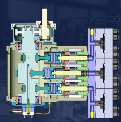
Our pumps designed for pumping various liquids, including chemically active, with temperatures from -15°C up to +450°C, kinematic viscosity not more than 8 cm/s, with the contents of solid non-abrasive particles up to 0.2% by weight and by size up to 0.2 mm.
