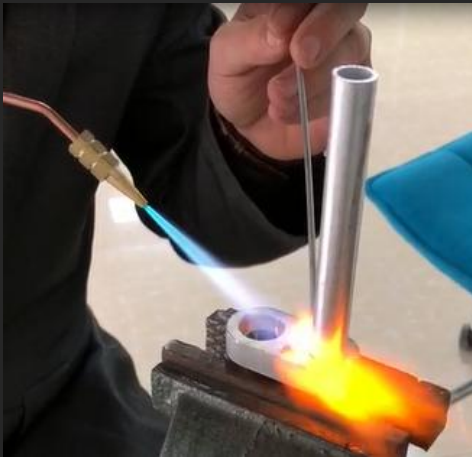
aluminium pipe welding
